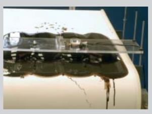
The metal particles are extracted in two flows, one in the centre, and one along the edge.
