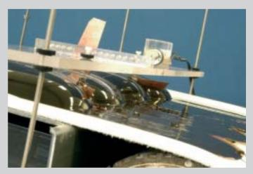
A separator vane inserted into the fluid down to 2 cm above the belt is used to separate the floating particles from those lying on the belt. The heavier particles move under the vane and drop off the end of the belt. The lighter particles float over the vane to hit a V-shaped ridge that carries them away to the side of the belt.
