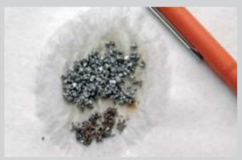
Separated particles of aluminium and copper
