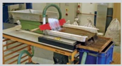
This test set-up devised by doctoral student Erwin Bakker was used for separating shredded PET from contaminants such as grit, glass, and metals. This test set-up also uses a magnetic fluid, but this time the fluid moves along with the PET particles. The contaminants remain behind at the bottom of the container. The PET particles are extracted by a screen
