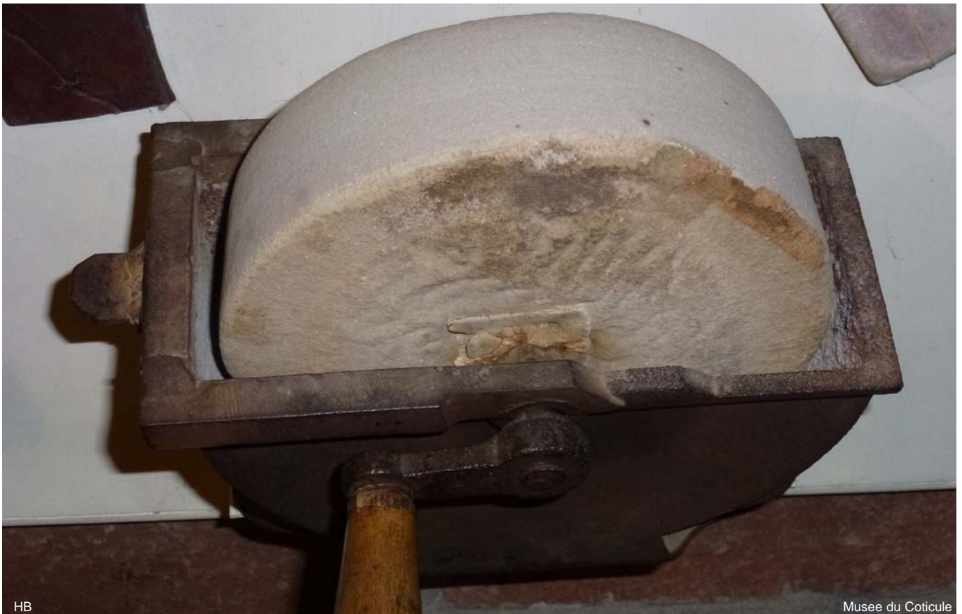
This bank stone is cut from a broken round grinding stone.
