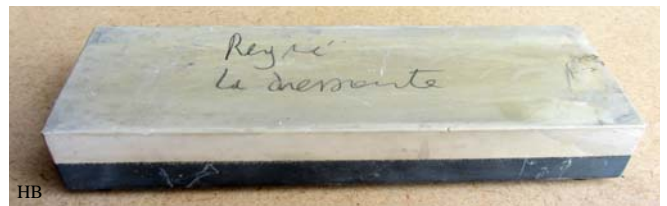
2 Samples from the Régné mine. La Verte has a scratch resistance of 1500 grams and the Dressante has a scratch resistance of 3000 grams, measured with a sclerometer.
