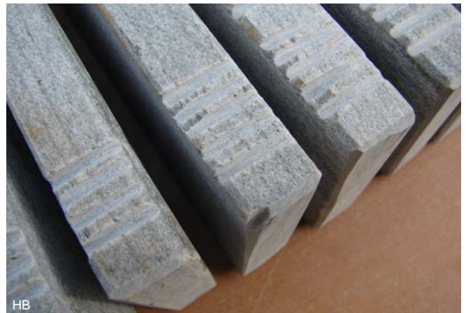
To keep the stones apart while burning, so they can be traced and keep good records, they are marked in a heat resistant manner.
