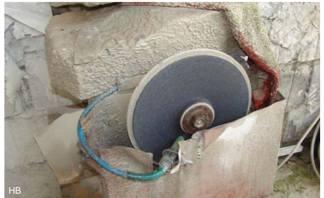
A slowly rotating SiC disc with water cooling for plane grinding and shape of the scythe stones.
