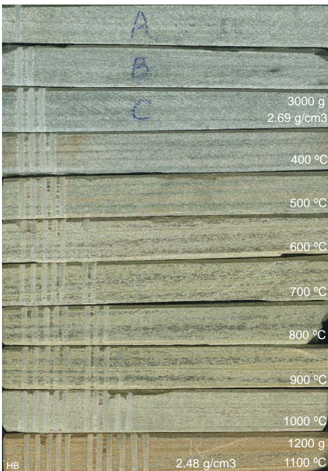
Started at 400 ° C and stopped at 1100 ° C.
