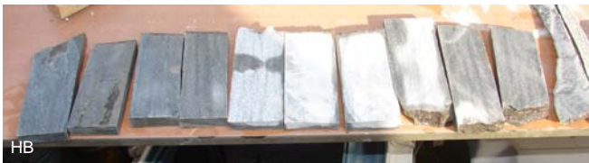
One side of the strips is ground flat to be able to clamp them against a stop which is set at 15 mm thickness. Now strips of 15 mm thick were sawn.
