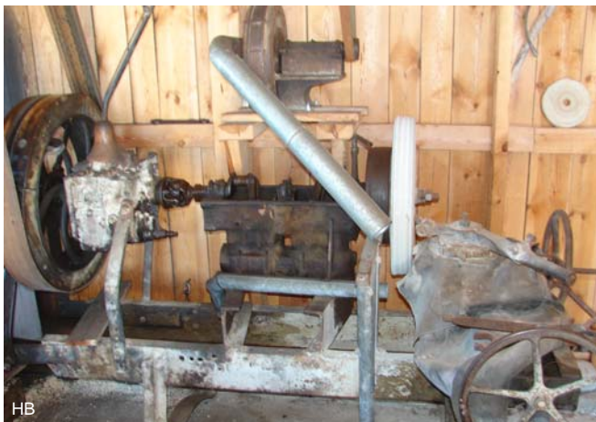
A lathe to turn grinding wheels. You take a gearbox and connects this via a universal joint to the crankshaft of an open engine block that is upside down. To the flywheel you attach your piece of work.
