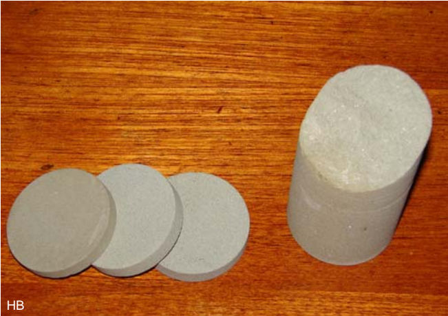
The slices are removed from the stone with a diamond drill and subsequently sawn into slices..
