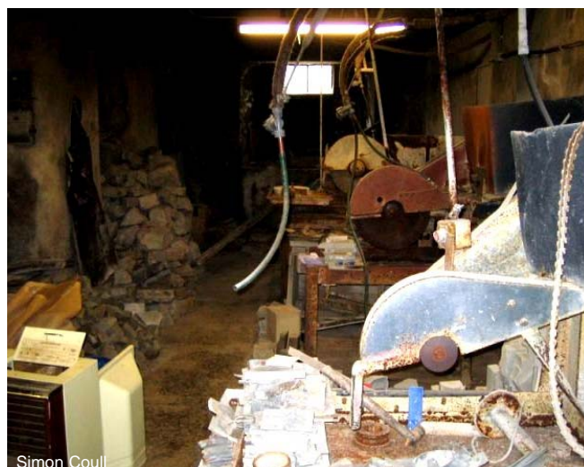
Since the integration of the firms, they were still in use on both sides, Heron's Mill was used to cut the blocks for hones, using diamond-fitting circular saws and the northern site is mainly used for facing, turning and polishing the whetstones.
