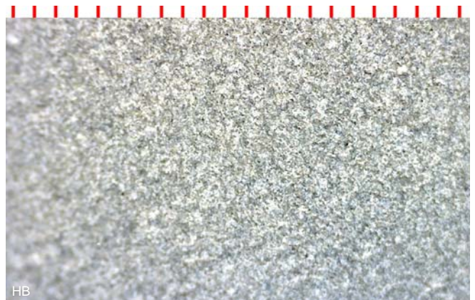
3 Polishing k 5000. The scale is 0.5 mm.
