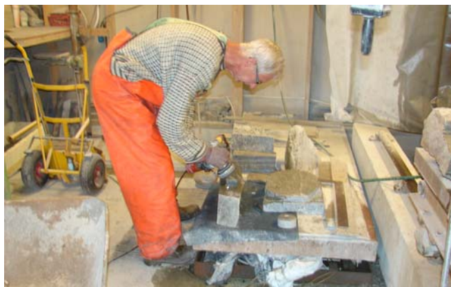
and finished with a water-cooled Flex with 100 grit.
