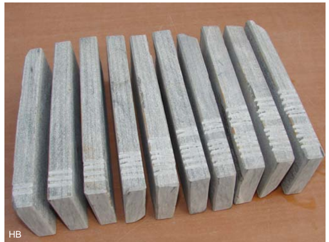
To keep the stones apart while burning, so they can be traced and keep good records, they are marked in a heat resistant manner.
