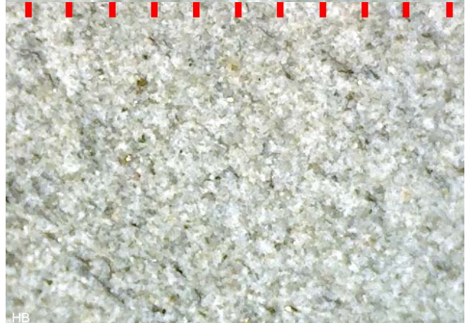
Micro 200x scale 0.5 mm. The top of a puck and the bottom of a fine bench stone.
