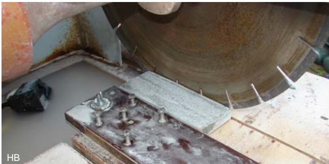
One side of the strips is ground flat to be able to clamp them against a stop which is set at 15 mm thickness. Now strips of 15 mm thick were sawn.
