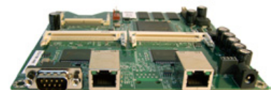
Dual PCI and Dual ethernetport. Makes smart-firewalling or 2,4 GHz and 5 GHz flexibility possible.
