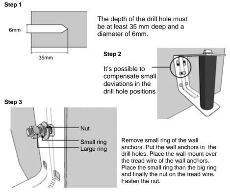
The wall mount is strong enough to hold a closed dish with a max. diameter of 1 meter.
