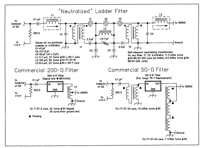
Figure 2—Example filter designs.
