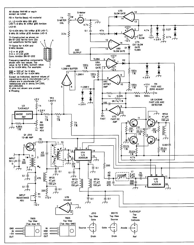
Figure 1—Schematic of the IF/AGC circuit. Where two values for a component are shown—one above and one below a short horizontal line—the upper value is for use at an IF of 9 MHz, the lower one for a 4.434-MHz IF. U8 and U9 are shown uncharacteristically here so as to provide a better understanding of circuit operation. FB-43-101 ferrite beads can be used.
