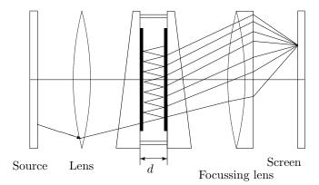
The width of the peaks at half height is given by  $\gamma = 4/\sqrt{F}$ . The finesse  $\mathcal{F}$  is defined as  $\mathcal{F} = \frac{1}{2}\pi\sqrt{F}$ . The maximum resolution is then given by  $\Delta f_{\min} = c/2nd\mathcal{F}$ .
