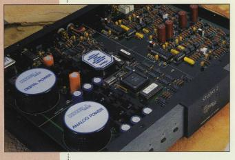
Separate power supplies are provided for the analog and digital circuitry. Digital circuitry is in the center of the unit with the analog stages at far right.
