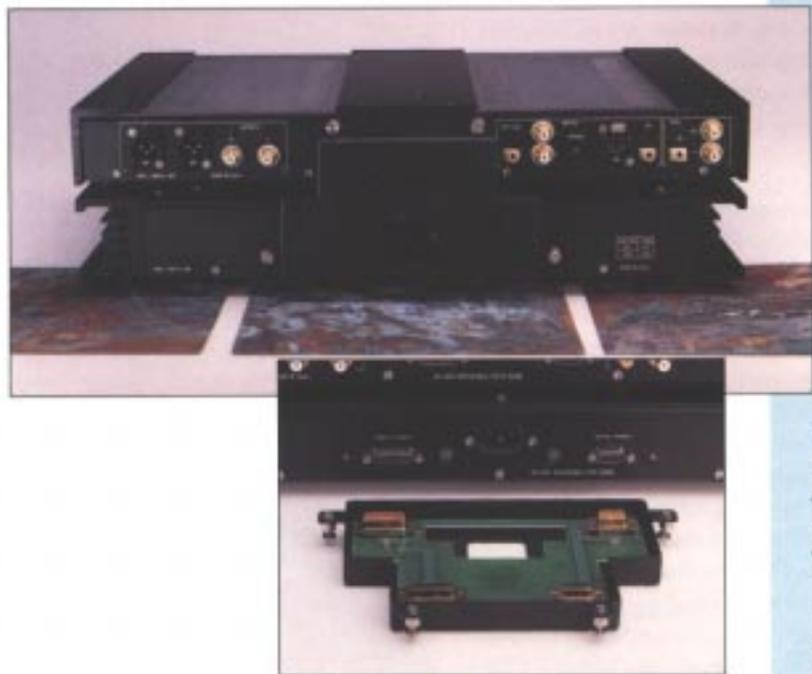
*The power supply and processor chassis are joined by a unique power coupler. A shielded circuit board transfers power and ground from the three supplies in a highly controlled manner. Eliminated by this technique are contaminations caused by conventional cables.*
