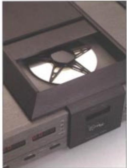
couples the disc to the transport in a comprehensive manner. Five arms contact the outer edges of the disc to insure uniform flatness. A quenched field magnet assembly achieves strong clamping force without affecting laser performance. The transport is fitted with a new spindle hub that interlocks with the stabilizer to prevent disc eccentricity.
