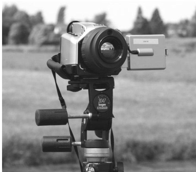
Figure 7. The thermo trace TH9100pro TIR camera used to map the emitted temperature of the dyke materials (photo taken during the summer field campaign).
