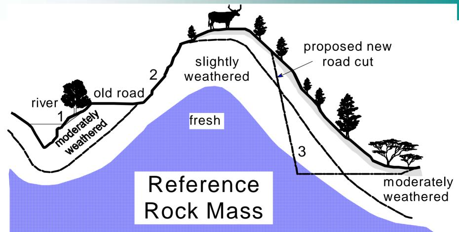
1: natural exposure made by scouring of river, moderately weathered; 2: old road, made by excavator, slightly weathered; 3: new to develop road cut, made by blasting, moderately weathered to fresh. Excavation specific parameters for the excavation which is used to characterize the rock mass
