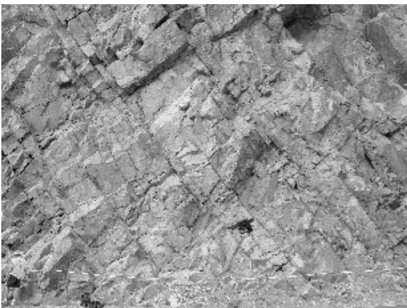
Figure 9. Colorado rock slope Photo 2. This exposure is around the corner from Photo 1 and is approximately 90° (perpendicular) to that exposure. Here the prominent large exposed surfaces visible in Figure 8 show on the image as dark lines that can be easily found with edge detection algorithms.
