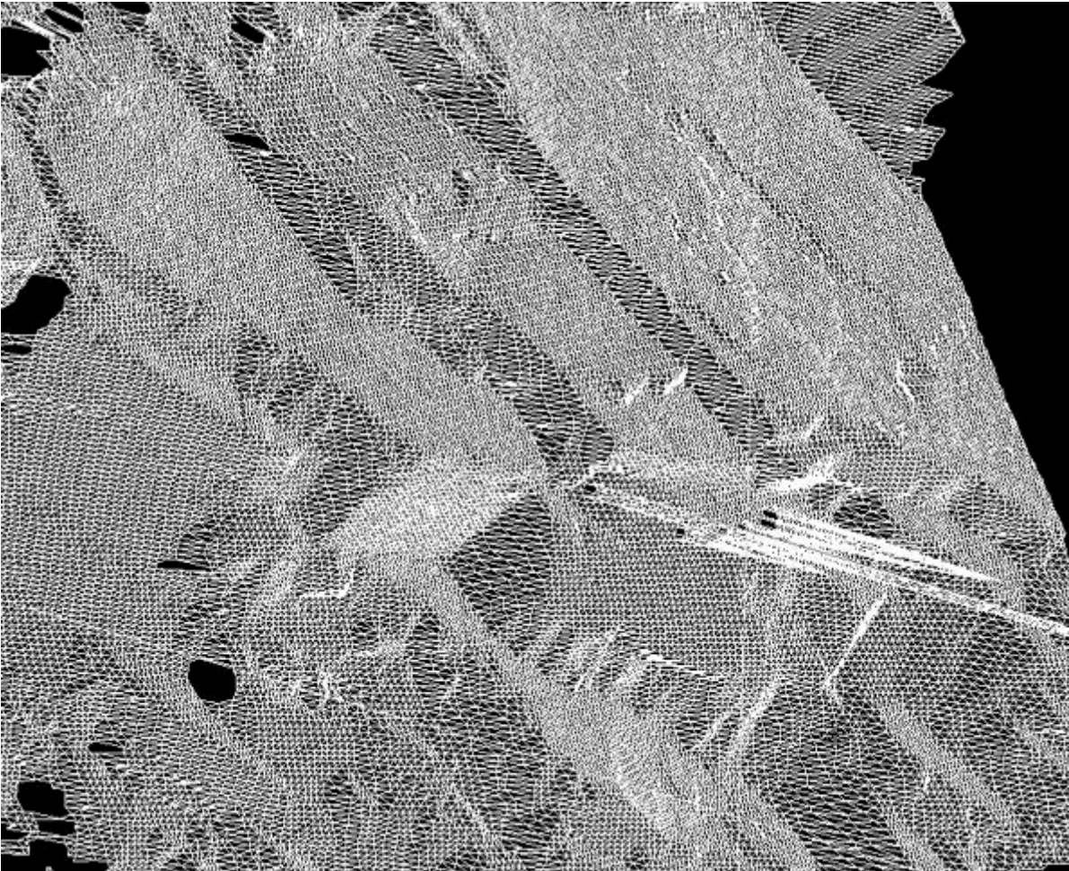
Figure 4. Detail of a triangulated mesh representing a small portion of a rock surface
