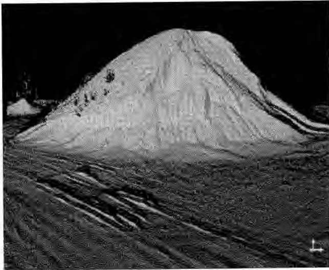
Fig. 3. Example of a 3D laser scan survey (point cloud with reflected intensity) of a sand pile. (From: Mensi, 2003).
