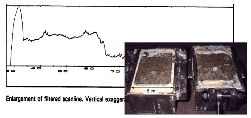
Laser roughness profile of sample in photo (after Baardman, 1993)
