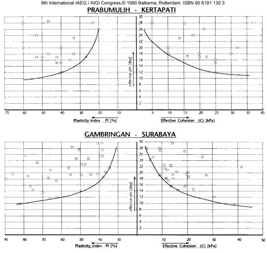
Figure 2. Examples Plasticity Index - effective phi and cohesion relation. (ch.7.4-4)
