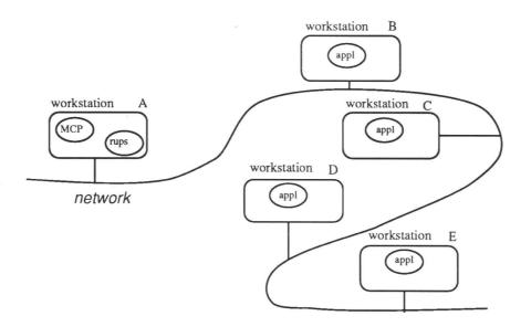
Figure 4: Mcp/rups and applications run on different machines in a network
