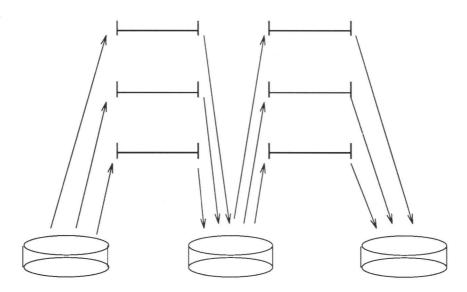
Figure 3: Each step reads data before and writes data afterwards
