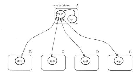
Figure 5: TCP/IP sockets provide the communications between mcp and the applications
