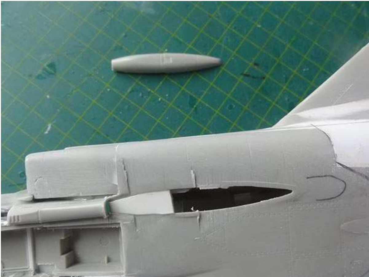
Some card was set and close the big gap. A 12 mm section was set in the middle and putty and sanding needed again!
