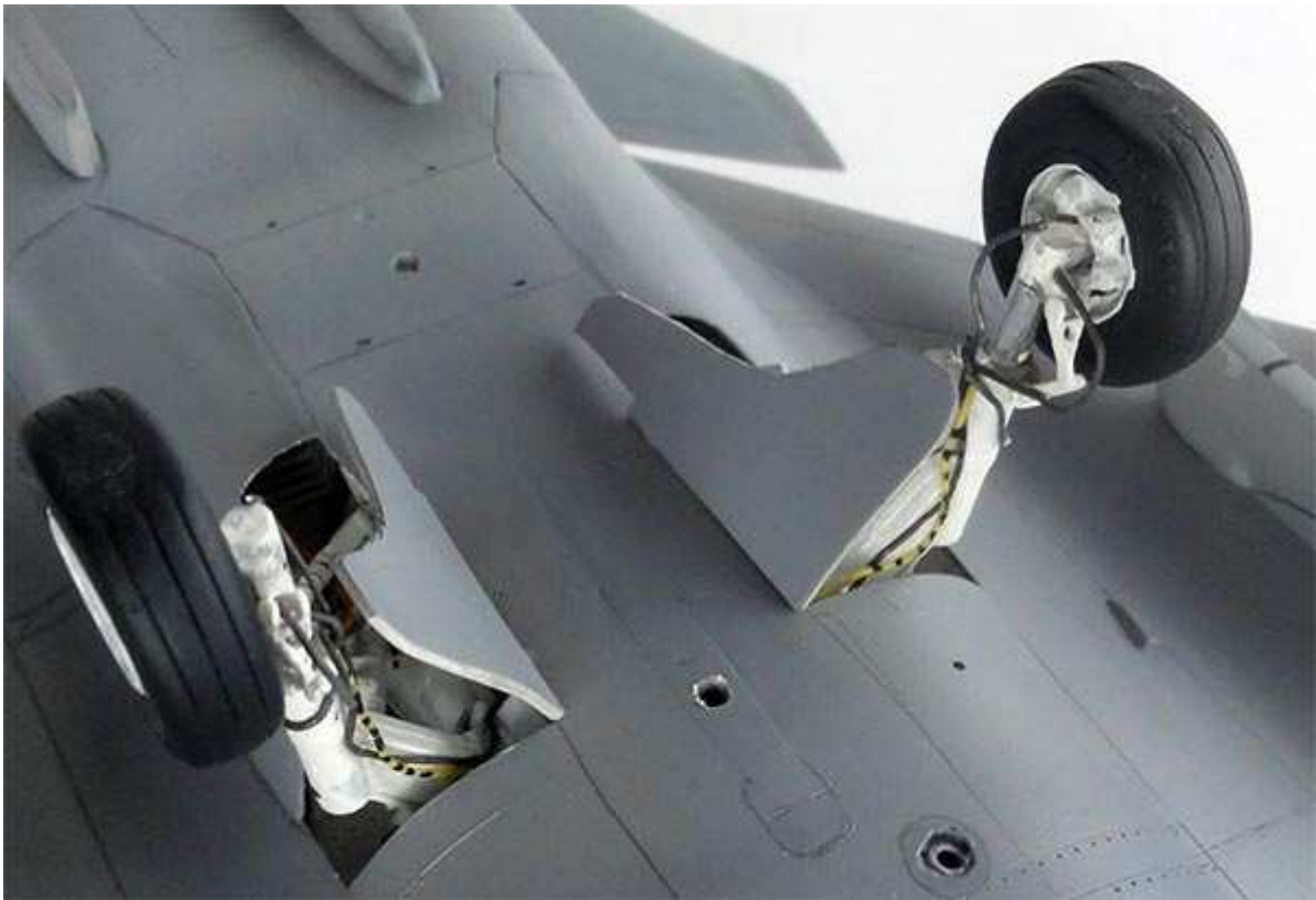
Note that the big main gear doors are in the “closed” position as seen on most parked Gripens. A few small curved gear doors were made from card (not seen here).
