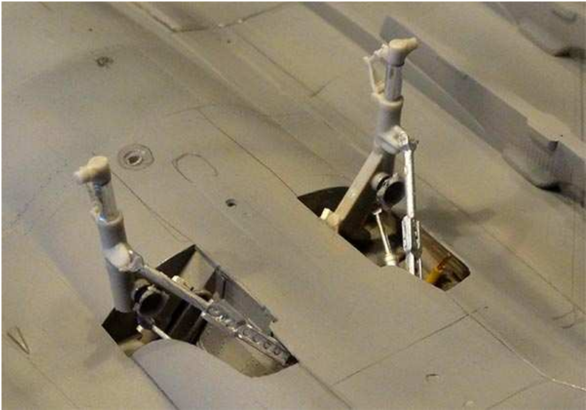
Note that the big main gear doors are in the “closed” position as seen on most parked Gripens. A few small curved gear doors were made from card (not seen here).
