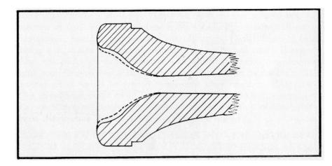
FIGURE 12: EFFECT OF CUP DIAMETER ON CUP VOLUME
