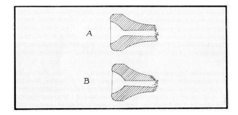
FIGURE 11: CUP SHAPES IN THE "SHOULDER-OF-THE-THROAT" AREA
