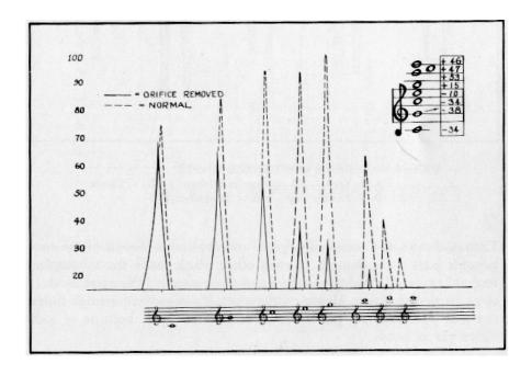
FIGURE 5: EFFECT OF EXTREMELY LARGE ORIFICE Intonation is shown as the change in cents caused by large orifice.
