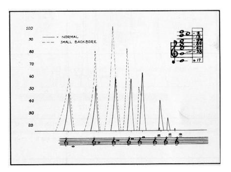
FIGURE 9: EFFECT OF SMALL BACKBORE Intonation is shown as the change in cents caused by small backbore.
