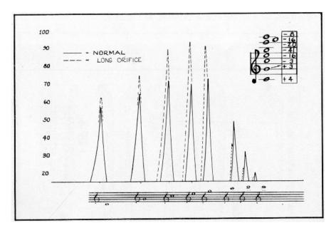
FIGURE 8: EFFECT OF LONG ORIFICE Intonation is shown as the change in cents caused by longer orifice.
