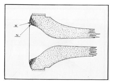
FIGURE 17: CONNSTELLATION MOUTHPIECE INNER RIM DIAMETER OPTIONS
