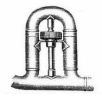
ABOVE we illustrate the tuning mechanism which is found on all "Victor" Cornets. This is a patented feature and while it is extremely helpful to the player it is also very simple and there is nothing to get out of order. Tuning is accomplished by turning the knurled wheel. Causing the slide to come out lowers the pitch, and causing the slide to go in raises the pitch.
