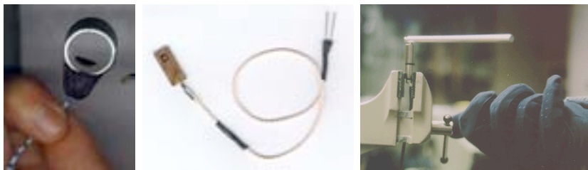
The Tactile Ring, a Tactor, and a mini motor controlled by SonoGlove
