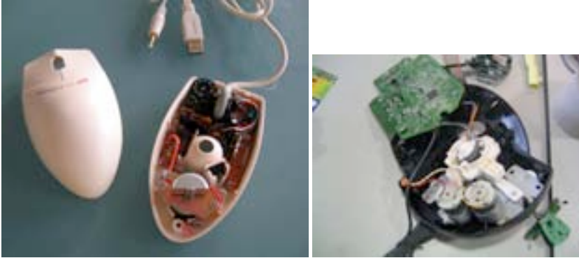
The AVB Tech mouse with eccentric weight (left) and a Logitech force-feedback joystick with motors (right)
