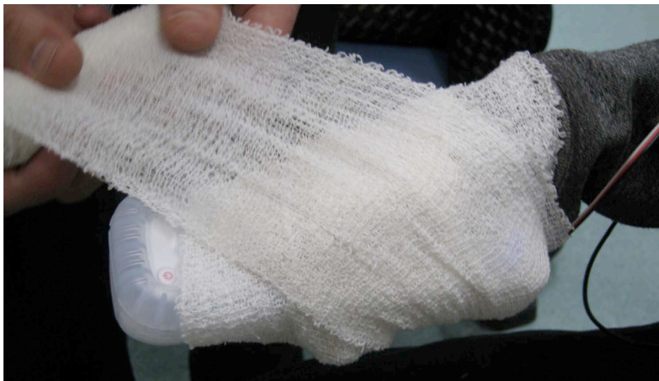
Figure 5. A Wii Remote strapped to the hand of the patient
