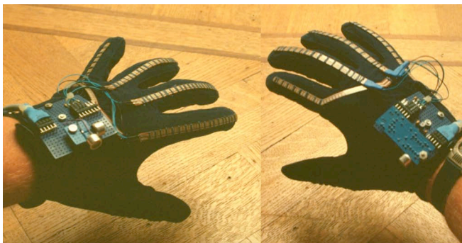
Figure 3. Instrumented gloves for musical performance.
