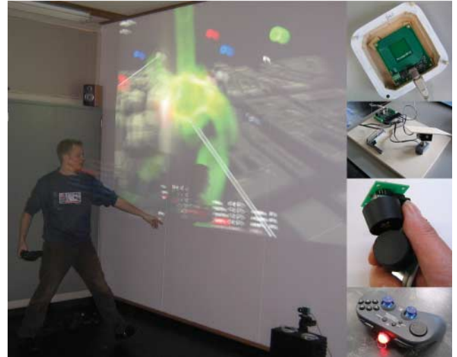
Figure 17. A selection of physical interaction modules, in use in the Protospace multi-user parametric design environment.
