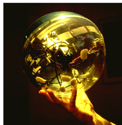
Fig. 28. Mercury tilt switches used in The hands II (left) and in a ball built for Ikaros van Duppen.
