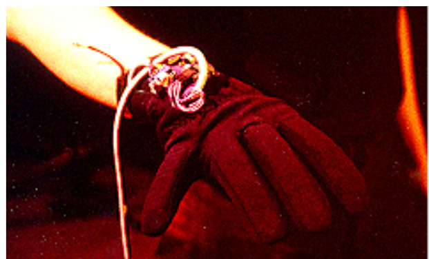
Fig. 20. Bend sensor for the Laser Bass, and glove built for Wart Wamsteker.
