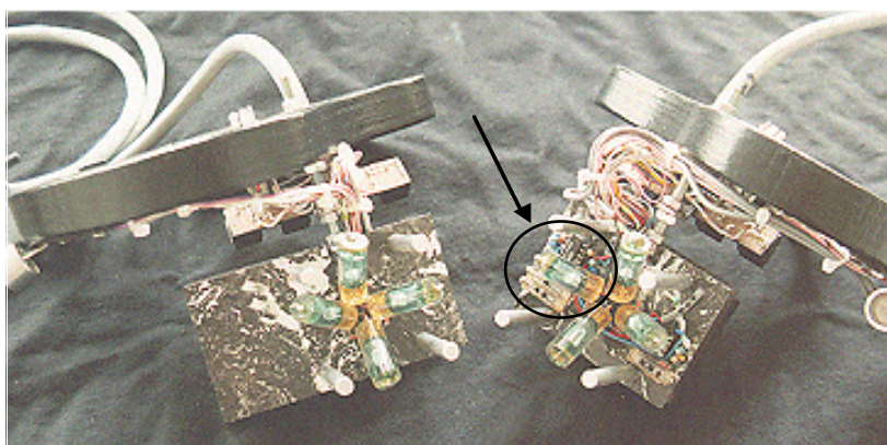
Fig. 28. Mercury tilt switches used in The hands II (left) and in a ball built for Ikaros van Duppen.
