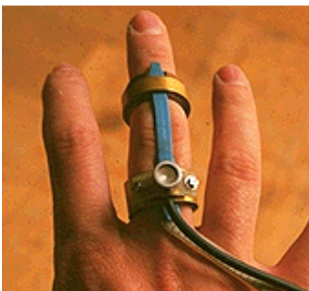
Fig. 20. Bend sensor for the Laser Bass, and glove built for Wart Wamsteker.
