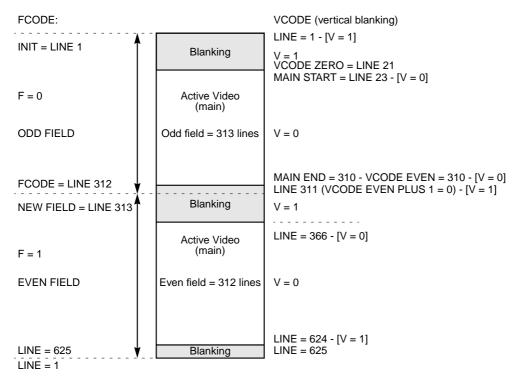
The last required parameter relating to the ITU-R BT.656 timing is the Fcode fields of Registers 303 and 305 (page 4-79). These bits are combined to specify the line number at which the field code bit changes. In general, the Fcode changes one line prior to the new field. For NTSC and PAL, this value is 265 and 312, respectively.
