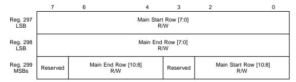
The host can write to these registers to program the start and end row numbers for the Main region on the display. The values entered are the number of lines from the start of a top or bottom field.
