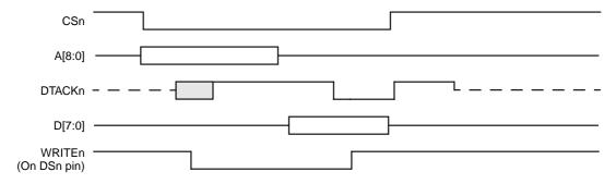
Figure 5.5 Intel Mode Read Timing
