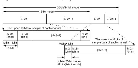
Figure 11.8 Linear PCM Audio Sample Syntax
