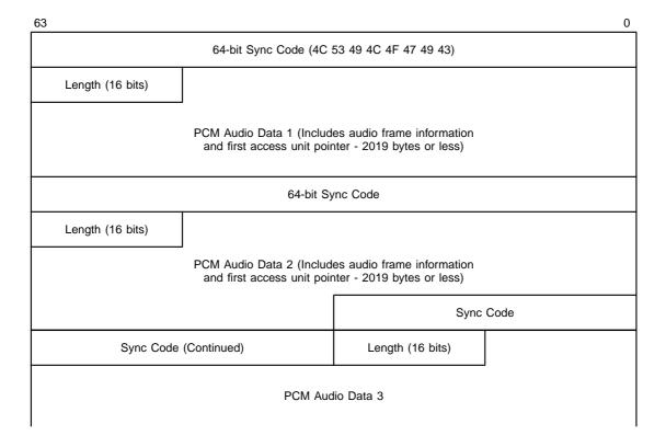
The Preparser adds a sync code and a data length field to the input Linear PCM packet header to provide the on-chip audio decoder with better error recovery features.
