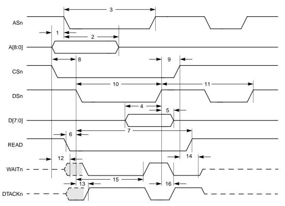
Figure 12.6 Host Read Timing (Motorola Mode)
