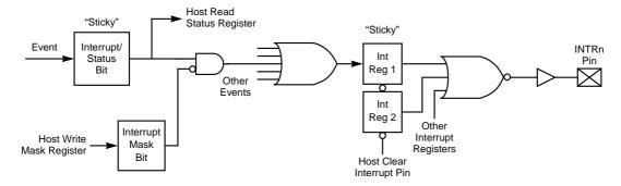
When the host detects INTRn asserted, it reads all of the interrupt/status registers to determine the cause of the interrupt and take any necessary action. The host read clears the interrupt/status bit but does not clear the associated IntReg. To deassert INTRn, the host must set the Clear Interrupt Pin bit in Register 6.
