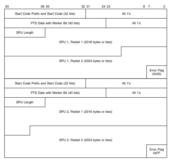
The SPU channel buffer stores the PTS data of the SPU header and the SPU packet data. SPU PTS data is stored with the start code prefix and the start code. Both have their upper bytes stuffed with 1's to form 64-bit words. If any error exists in an SPU, the error flag in the last packet is set to 0xFF. If there is no error, the error flag is left at 0x00. If there is an error between the SPU Length field and the actual SPU length, the
