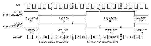
Note: S means sign-extension (0 for positive PCM values, 1 for negative PCM values).
