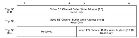
These registers contain the current write pointer address of the Video ES channel buffer. The LSB should be read first, since this captures the next significant byte and MSB in Registers 97 and 98. These should then be read immediately to ensure that the correct captured value is read. When set, the most significant bit (bit 3 of Register 98) indicates that the write pointer has wrapped around from the end address to the start address of the buffer.
