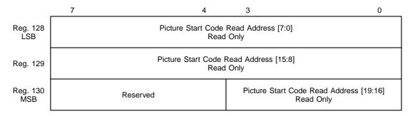
These registers contain the address of the video channel read pointer captured at the time that a picture start code is decoded from the bitstream by the decoder. When set, the most significant bit (bit 3 of Register 130) indicates that the read pointer has wrapped around from the end address to the start address of the buffer.
