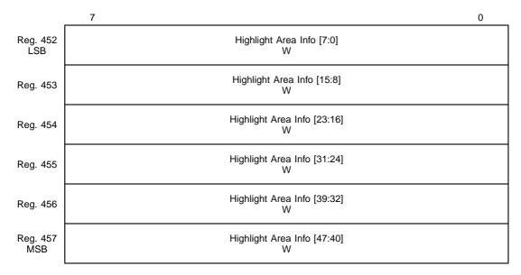
These registers supply the area information for highlight. The bit allocation is the same as the button position information in the *DVD Specifications for Read-Only Disc.*
