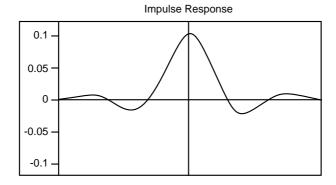
The scale factor of the interpolator is the ratio between the widths of the source image and the target image in 1/256th of a pixel increments. The interpolator calculates the subpixel position to within 1/256th of a pixel and chooses one of the eight filter banks closest to the calculated location. The filter integrates a raster mapper that increments by n/256 each output pixel.
