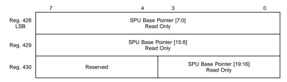
These registers contain the SPU base pointer word address in which SPUSZ (SPU size) is located.
