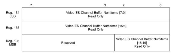
These registers contain the number of items (64-bit words) remaining to be read in the Video ES channel buffer. The LSB should be read first since this captures the next significant byte and MSB in Registers 135 and 136. These should then be read immediately to ensure that the correct captured value is read.
