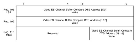
The host can write a Video ES channel buffer address in these registers to be compared with the current read pointer address of the Video ES channel buffer. When the current read pointer address matches the contents of the registers and the chip is in the Video Read Compare Mode (Register 69, bit 0 set, page 4-22), the DTS Video Event Interrupt bit (Register 2, bit 7, page 4-7) is set and, if the interrupt is not masked, the INTRn output signal is asserted.
