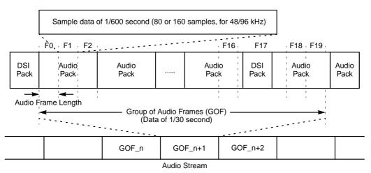
Figure 11.7 Linear PCM Packet Syntax
