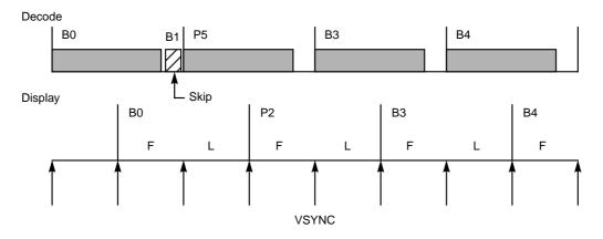
Case 2: One-time skip B picture causing display freeze
