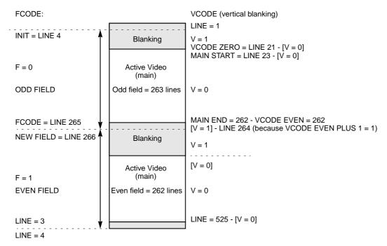
The Vcode Zero field of Register 303 (page 4-79) specifies the line number at which the vertical blanking bit in the EAV code should change from one to zero. This value is dependent on the particular timing system. It is typically set to 21 for NTSC and PAL.
