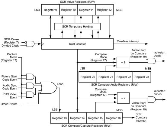
In the Capture Mode, the host can select an event in the bitstream to use for capturing the value of the SCR counter. When the preparser in the chip detects the selected event, the SCR counter value is loaded into the SCR Compare/Capture registers. The host can read these registers at some later time to determine exactly when the event occurred. The following events can be selected for SCR capture:
