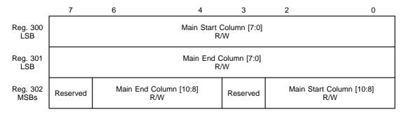
The host can write to these registers to program the start and end column numbers for the Main region on the display. The values entered are the number of system clocks from the horizontal sync signal.
