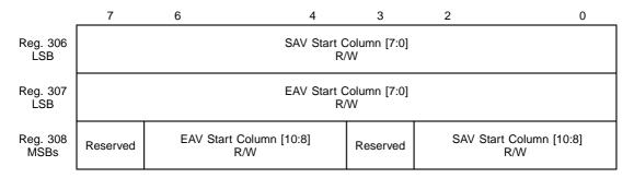
The host can write to these registers to define the start of SAV and EAV in terms of the number of system clocks from the horizontal sync.
