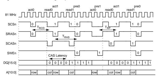
Figure 7.3 SDRAM Timing Requirements for Writes
