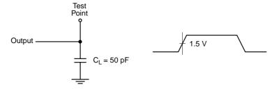
For 3-state outputs (see Figure 12.2), timing measurements are made from the point at which the output turns ON or OFF. An output is ON when its voltage is greater than 2.4 V or less than 0.4 V. An output is OFF when its voltage is less than 2.4 V or greater than 0.4 V.
