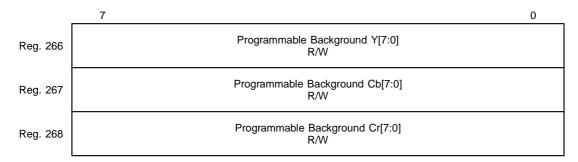
When the Force Video Background Mode (bits 6 and 7 in Register 265) is 0b10, the Y, Cb, and Cr values for the background are specified in Registers 266, 267, and 268, respectively. The default values (i.e., values in the register at startup/reset) are Y=35, Cb=212, and Cr=114. These values correspond to 75% Amplitude, 100% Saturated Blue.
