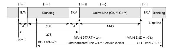
The vertical line count is used for positioning the display areas vertically and it is initialized at the new field boundary. The vertical line count is used to compare with the start and end rows of each display area and increments with each horizontal sync. In some timing systems (i.e., NTSC), the vertical line count does not initialize to a value of one. For NTSC and PAL systems, the Vline Count Init value in Register 282 (page 4-75) should be programmed to four and one, respectively.
