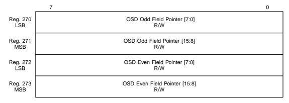
The host can program the addresses of the OSD Odd/Even Field Pointers into these registers. The addresses are in 64-byte resolution.
