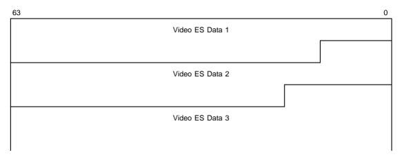
Figure 6.21 shows a map of the Navi Pack Channel Buffer. The buffer stores all PCI and DSI packet data of private\_stream\_2. PCI and DSI packet data is word aligned after the last PCI/DSI data stored.
