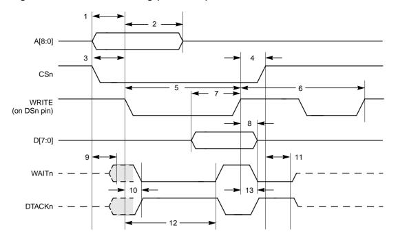
Figure 12.8 Host Read Timing (Intel Mode)
