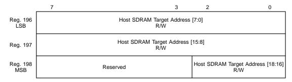
For a host write to SDRAM, the host must write the starting SDRAM address in this register. This address is automatically incremented after eight bytes are transferred to SDRAM through Register 195 and the internal, 8 x 64, write FIFO. The host should update the SDRAM target address only when the write FIFO is empty.
