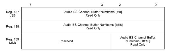
These registers contain the number of items (64-bit words) remaining to be read from the Audio ES channel buffer to the selected Audio Decoder. The LSB should be read first, since this captures the next significant byte and MSB in Registers 138 and 139. These should then be read immediately to ensure that the correct captured value is read.
