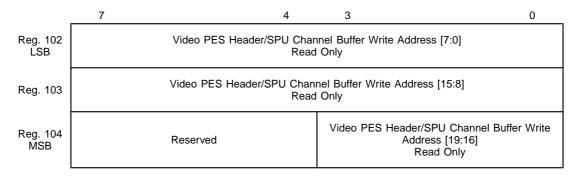
These registers contain the current write pointer address of the Video PES Header/SPU channel buffer. The LSB should be read first, since this captures the next significant byte and MSB in Registers 103 and 104. These should then be read immediately to ensure that the correct captured value is read. When set, the most significant bit (bit 3 of Register 104) indicates that the write pointer has wrapped around from the end address to the start address of the buffer.
