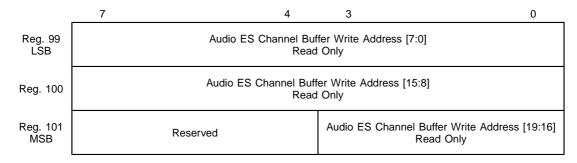
These registers contain the current write pointer address of the Audio ES channel buffer. The LSB should be read first, since this captures the next significant byte and MSB in Registers 100 and 101. These should then be read immediately to ensure that the correct captured value is read. When set, the most significant bit (bit 3 of Register 101) indicates that the write pointer has wrapped around from the end address to the start address of the buffer.
