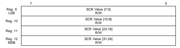
These registers contain the current value of the System Clock Reference (SCR) Counter. The host must read Register 9, the LSB, first. This captures the upper 24 bits and writes them into Registers 10, 11, and 12. The host must set the SCR Pause bit in Register 8 before writing to these registers.
