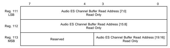
These registers contain the current read pointer address of the Audio ES channel buffer. The LSB should be read first, since this captures the next significant byte and MSB in Registers 112 and 113. These should then be read immediately to ensure that the correct captured value is read. When set, the most significant bit (bit 3 of Register 113) indicates that the read pointer has wrapped around from the end address to the start address of the buffer.
