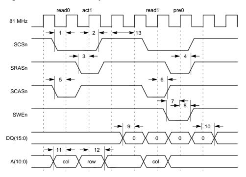
Figure 12.4 SDRAM Write Cycle
