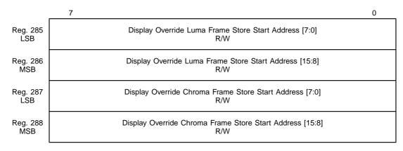
The host can write to these registers to override the display picture luma and chroma frame store start addresses when the Display Override Mode (Register 265, bits 4 and 5, page 4-68) is set to Frame (0b01) or First Field Only (0b10).
