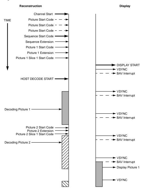
Figure 8.3 Time Line for Field Picture
