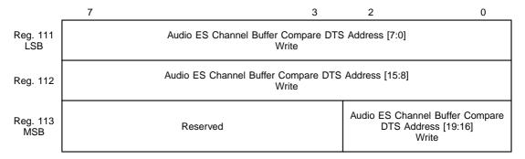
The host can write an audio channel address in these registers to be compared with one of the current read pointer addresses of the Audio ES channel buffer. When the selected current read pointer address matches the contents of the registers and the chip is in one of the Audio Read Compare modes (Register 69, bits 1 and 2, page 4-23), the DTS Audio Event Interrupt bit (Register 2, bit 6, page 4-7) is set and an interrupt is generated, if not masked, by asserting the INTRn output signal.
