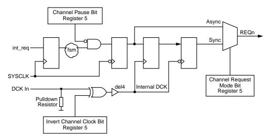
The internal request (int\_req) signal is generated by the channel input FIFO controller on the L64020 and indicates available room in the on-chip buffers and the SDRAM channel buffers. The internal request signal
