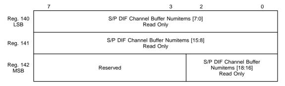
These registers contain the number of items (64-bit words) remaining to be read from the Audio ES channel buffer to the MPEG or Dolby Digital S/P DIF Formatter. The LSB should be read first since this captures the next significant byte and MSB in Registers 141 and 142. These should then be read immediately to ensure that the correct captured value is read.
