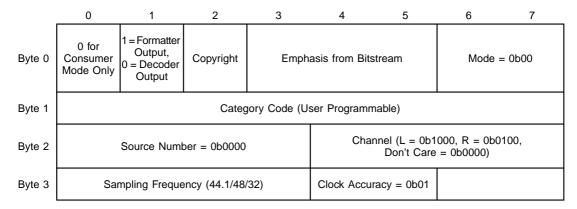
The host can overwrite the Copyright bit, the Emphasis bits, and Category Code by setting the associated overwrite bit in Registers 365 (page 4-101) and 366 (page 4-102), and writing to the Emphasis bit, Copyright field, or Category field in Register 367. The remaining bits and fields of the channel status bytes are fixed or filled in by the S/P DIF Interface as shown in Figure 11.21.
