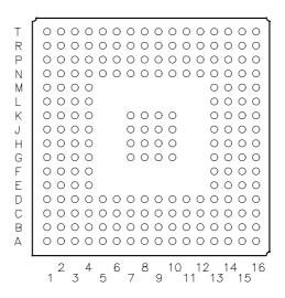
Table 12.13 208-Pin mini-BGA Array Signal Assignments
