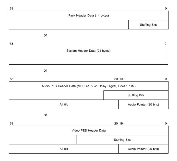
Figure 6.16 SPU Channel Buffer Map for DVD Streams
