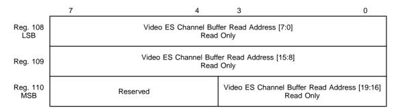
These registers contain the current read pointer address of the Video ES channel buffer. The LSB should be read first, since this captures the next significant byte and MSB in Registers 109 and 110. These should then be read immediately to ensure that the correct captured value is read. When set, the most significant bit (bit 3 of Register 110) indicates that the read pointer has wrapped around from the end address to the start address of the buffer.
