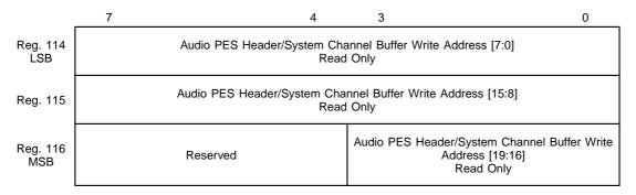
These registers contain the current write pointer address of the Audio PES Header/System channel buffer. The LSB should be read first, since this captures the next significant byte and MSB in Registers 115 and 116. These should then be read immediately to ensure that the correct captured value is read. When set, the most significant bit (bit 3 of Register 116) indicates that the write pointer has wrapped around from the end address to the start address of the buffer.
