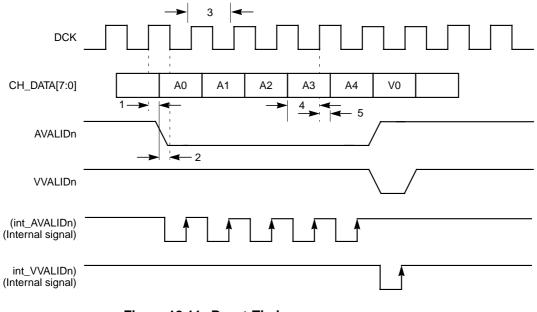
Figure 12.11 Reset Timing
