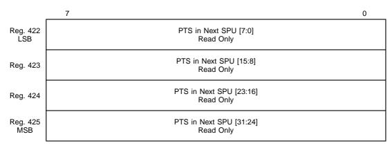
Registers 422 through 425 contain the PTS in the next unit. If the next unit is not in the channel buffer, this value is equal to the PTS in Current SPU.
