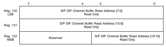
These registers contain the current address of the S/P DIF (IEC958) read pointer in the Audio ES channel buffer. The LSB should be read first since this captures the next significant byte and MSB in Registers 121 and 122. These should then be read immediately to ensure that the correct captured value is read. When set, the most significant bit (bit 3 of Register 122) indicates that the read pointer has wrapped around from the end address to the start address of the buffer.
