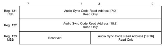
These registers contain the address of the audio channel read pointer captured at the time that an audio sync code is decoded from the bitstream by the Audio Decoder. When set, the most significant bit (bit 3 of Register 133) indicates that the read pointer has wrapped around from the end address to the start address of the buffer.
