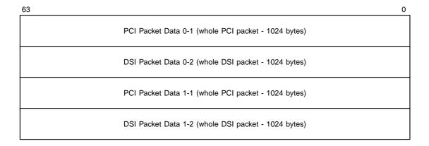
Figure 6.22 shows a map of the Data Dump Channel Buffer.
