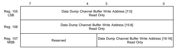
These registers contain the current write pointer address of the data dump channel buffer. The LSB should be read first, since this captures the next significant byte and MSB in Registers 106 and 107. These should then be read immediately to ensure that the correct captured value is read. When set, the most significant bit (bit 3 of Register 107) indicates that the write pointer has wrapped around from the end address to the start address of the buffer.
