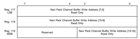
These registers contain the current write pointer address of the Navi Pack channel buffer. The LSB should be read first, since this captures the next significant byte and MSB in Registers 118 and 119. These should then be read immediately to ensure that the correct captured value is read. When set, the most significant bit (bit 3 of Register 119) indicates that the write pointer has wrapped around from the end address to the start address of the buffer.
