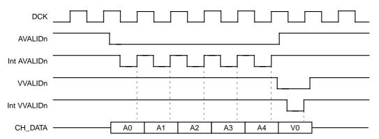
The constraints on synchronous valid signal mode are:
