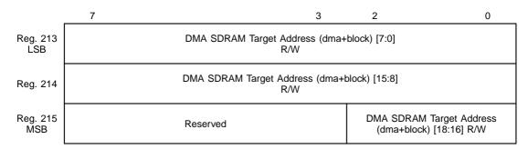
During DMA Write and Block Move, the DMA SDRAM Target Address is the starting address where future DMA writes will take place. This address is automatically incremented after a 64-bit word is transferred to SDRAM from the internal 8 x 64 write FIFO. The DMA SDRAM Target Address should be updated by the host only when the write FIFO is empty.
